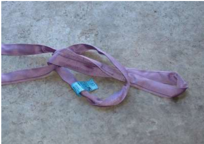
Join one long sling to a short sling as shown. This extended sling is used at the bow.
