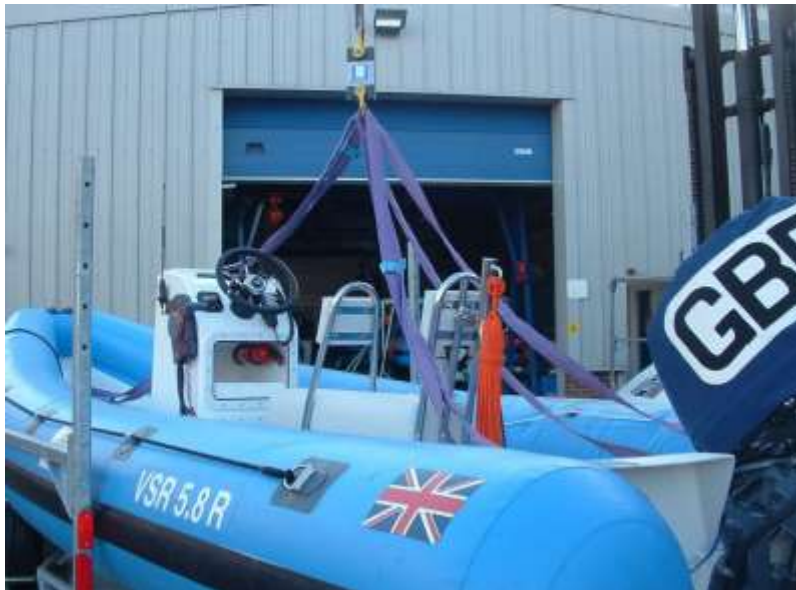
Lift the boat as shown. Be careful to make sure the slings are not caught under the throttle box or steering wheel.
