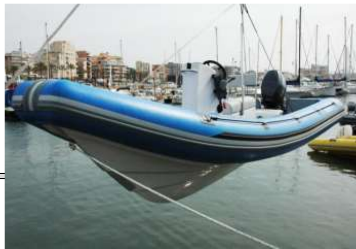
Lift the boat as shown. Be careful to make sure the slings are not caught under the throttle box or steering wheel.
