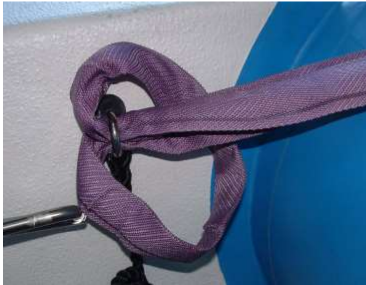
Fit the slings to the two eyes in the stern and one eye in the bow as shown.
